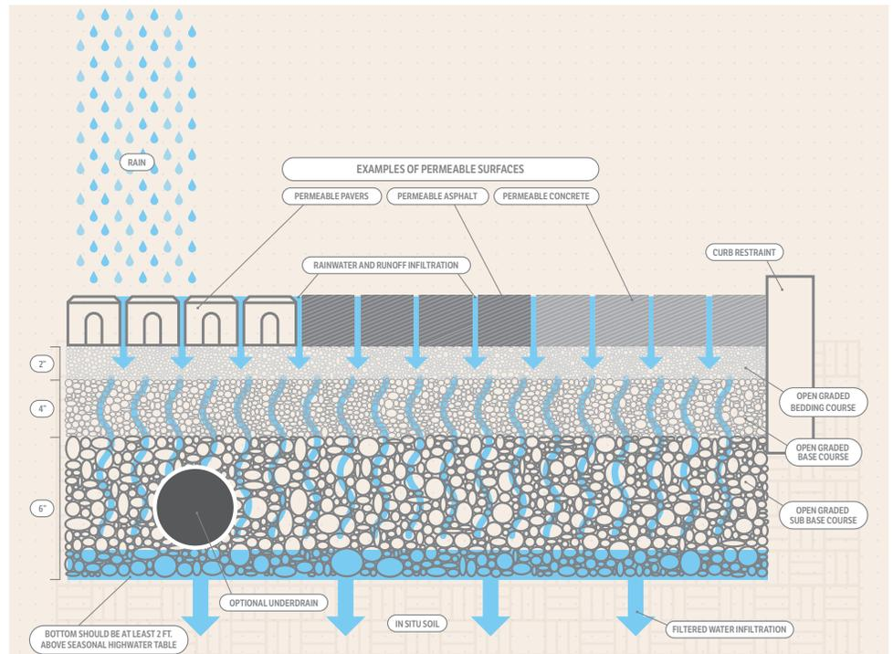
**Figure 9.** Illustration of a typical permeable pavement system
