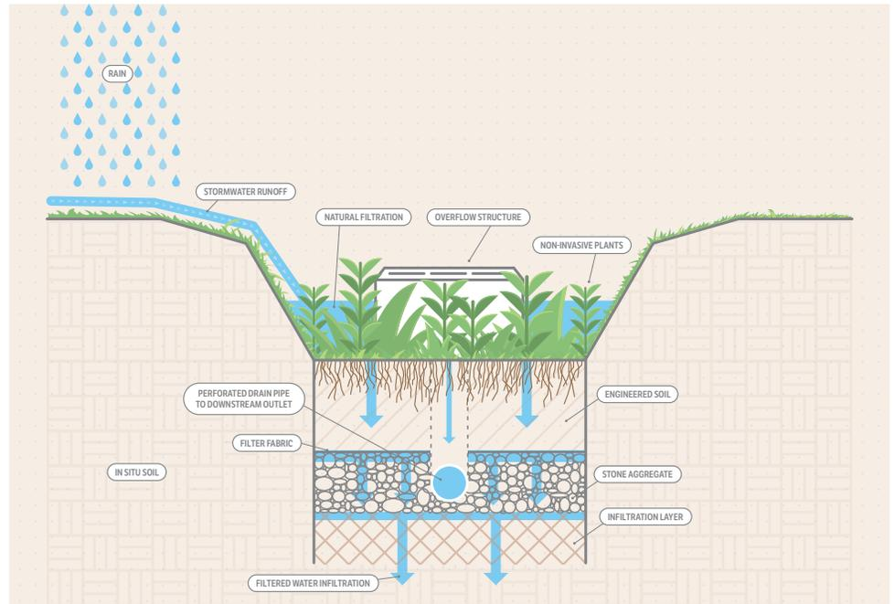
**Figure 6.** Illustration of a typical bioswale system
