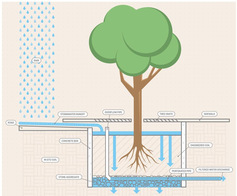
Figure 4. Illustration of a typical tree box system
